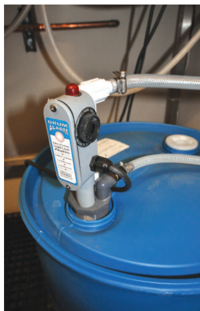
Pick-up tube with low level indicator
