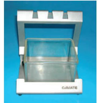
TPX container for keeping prongs submerged in sterilization solution
